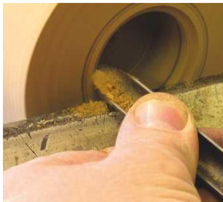
▲ Pic.5 He is opening the top of the hole 10mm wider and the same depth. This is to allow him to cut the fingers or spikey top on the candle holder
